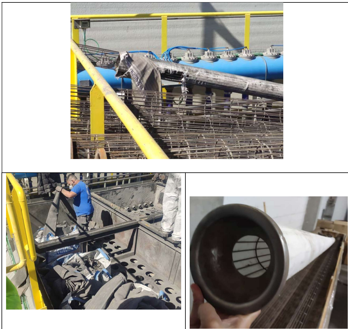
Figure 52 Old and new bag filters
